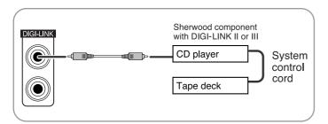
Connect this jack to the DIGI-LINK jack of the external Sherwood component that uses the DIGI-LINK II or III remote control system.
